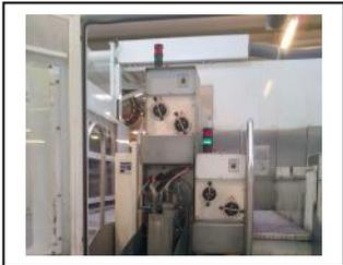
On fixed print units shearing and crushing injuries when lowering the print unit into the operating position.
