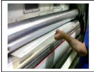
On print units in-running nips and entanglement in rotating print rollers during setting and attaching and removing stereos.
